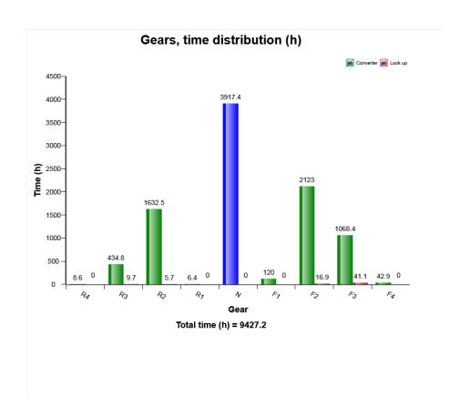
The graph describes the distribution of the usage of the different gears, expressed as total running time for each gear..
