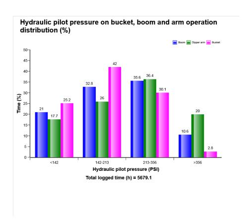
The diagram describes the distribution of hydraulic pilot pressure in specified operation
