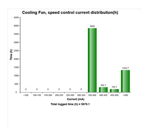
The diagram describes Hydraulic Cooling fan speed control, Current (mA) distribution, on fan speed Control..
