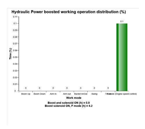
T he diagram describes Power boosted operating time distribution, when main relief pressure increases on working operation modes. In this diagram, the sum of time (%) of each working operation mode can exceed 100%. It means that customer has been operated several working operations at the same time.
