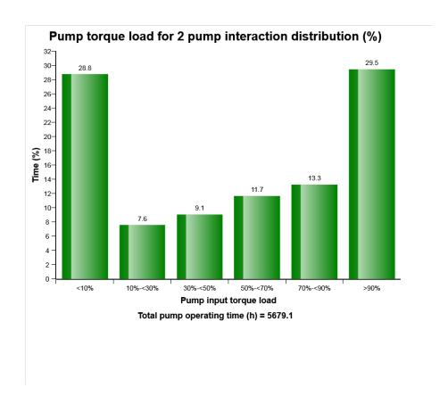
This is to see total torque load distribution of 2 pumps when it operates 2 pumps at the same time.
