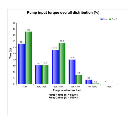
The diagram describes Pump torque load of 2 Pumps distribution.
